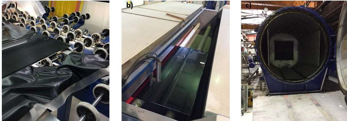
Figure 1. Lamination process for PVB laminated glass panels: a) assembly of composite panel, b) passing through oven and rollers to form initial bond and c) placement in autoclave to form the final product (Courtesy of Romvos Glass S.A.).
